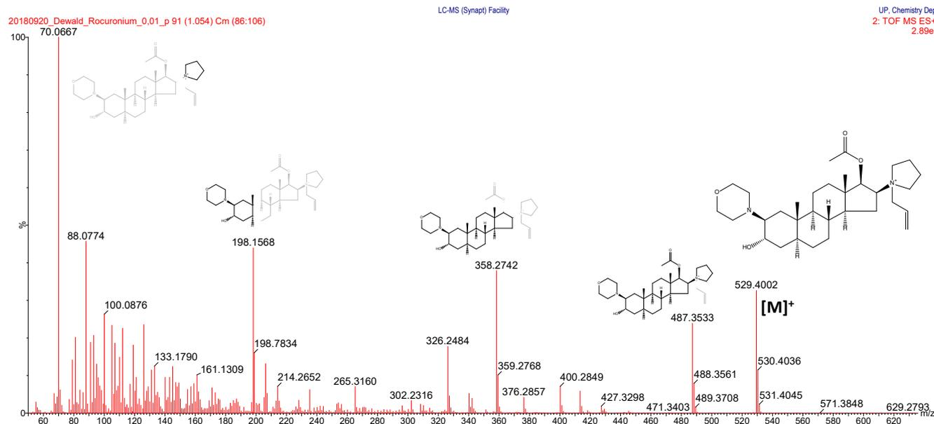
Figure 2: High energy mass spectrum of rocuronium (529.4002 m/z) ( $[M]^+$  salt counterion) giving the MS/MS fragmentation pattern of the compound for qualitative confirmation
